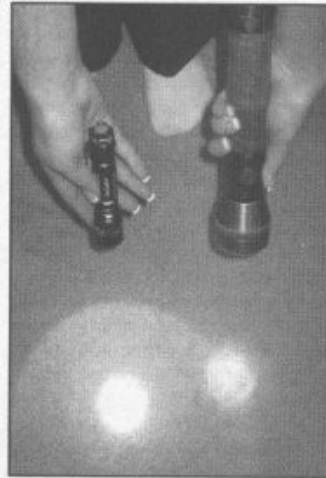
The Remington light on left uses two CR123 batteries and really outshines the incandescent 5 "D" cell light on the right with new batteries. Notice how much whiter and brighter the LED light is compared to the regular light.
